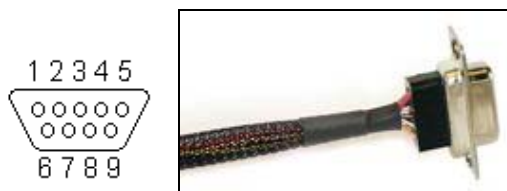
Figure 3: DB-9 Female Cable Connector (Rear View)
